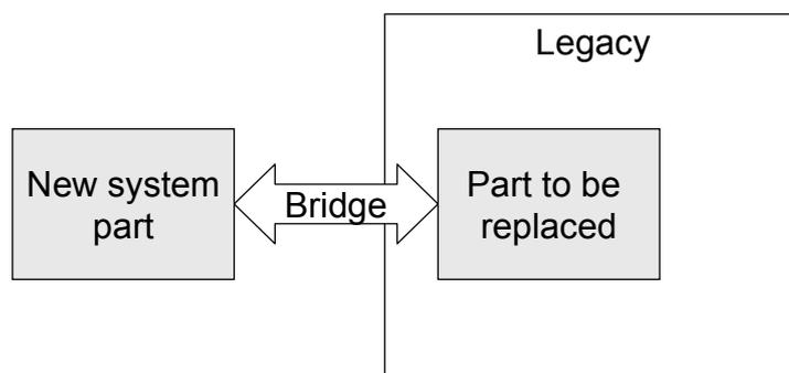
As mentioned in the solution you have the *legacy*, which contains a *part to be replaced*. In order to replace this part with a new system, you install the *new system part* and connect it to the *legacy's part to be replaced* using a *bridge*.
