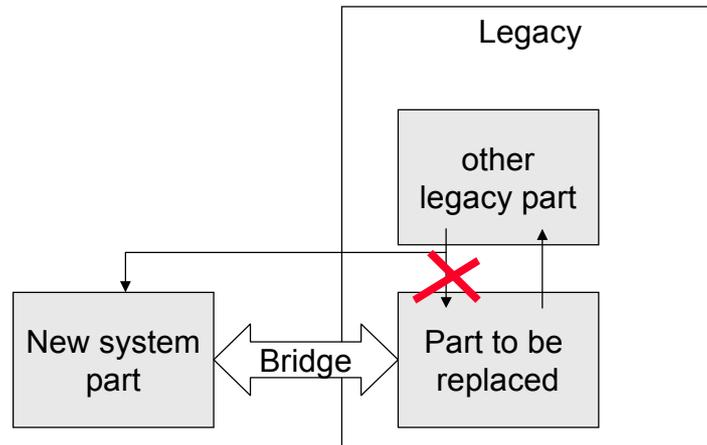
The above figure shows that you have to watch especially inbound data traffic into the *part to be replaced*. You need to redirect all of this traffic to the *new system part*. Either via the *bridge* or directly online. On the other hand, any *other legacy part* can work on in an undisturbed fashion as the read access to data entered in the *new system part* need not be redirected to the *new system part* but the code may still access the *part to be replaced*.
